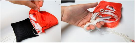
Grab the lines and wind them round your fingers till it looks like an 8 in order to store the lines in the container. Then house the lines inside the container just in front of the parachute's trailing edge.
