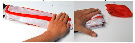
The trailing edge of the parachute should be positioned on the opening side of the container.
