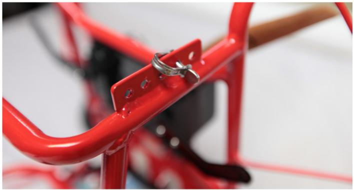
The trike features numerous holes to adjust the way you can fasten the wing risers. How do we define what hole has to be used?
