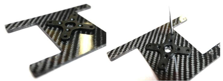
Use a sharp tool to mark where you are going to drill according to the crosspiece geometrical structure. Then drill trough the locking plate using a drill.
