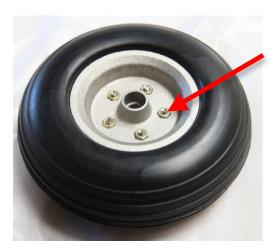
Insert the on spacer ring (5mm diameter). the other side of the rim. Insert the nuts on the other side of the rim. Screw the screws and the nuts firmly.
