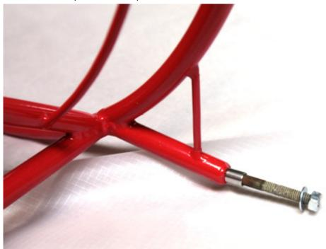
Unscrew the nut and remove the washer. Then insert the wheel and screw the washer and the nut back. Don't screw it too hard to let the wheel rotate around the axle. As usual, please secure the nut using thread sealant or some Loctite super glue.
