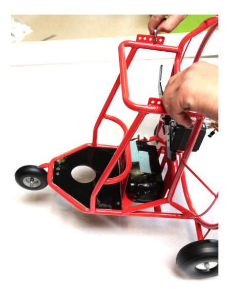
The battery has to be placed the way shown on the picture above thus positioning the center of gravity properly. Doing so will enable you to bring up to 3 kgs onboard using the front side of your trike.
