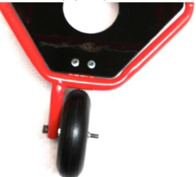
Unscrew the Nylstop nut and remove the washer. Then insert the wheel and screw the washer and the Nylstop nut back. Make sure the wheel can turn freely and doesn't rub against the frame.
