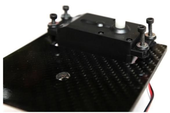
Insert the 4 HSHC screws and their washers. Put the servomotor on the locking plate. Do the exact same thing for the 2nd servomotor.
