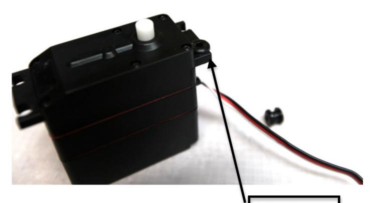
Put the 4 rubber eyelets in place
