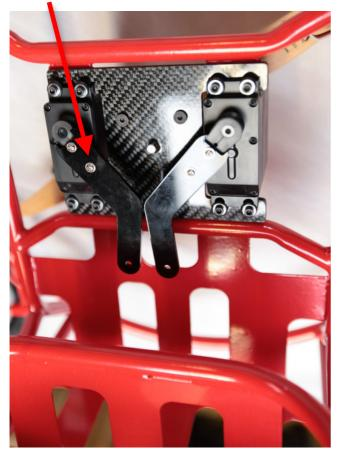
You can now put the arms onto the servomotors.
