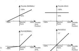
curve E.g. set the throttle curve in IDLE1 / IDLE2 / IDLE3 mode to 65% / 75% / 85% respectively to experience different RPM, and then adjust the value according to the actual situation or preference. 5) As the battery voltage decreases & the pitch of main rotor blades varies in flight, so we recommend setting the throttle curve between 60%~85% (here we strongly suggest not set the value exceeds 85%) or
