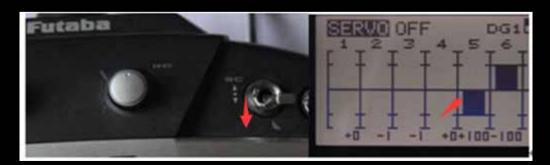
Check channel if is reversed (AILE, ELEV, RUDD, CH5, CH6) CH6, Up position, 900US< CH6 < 1520US</li>
