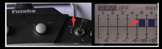
Check channel if is reversed (AILE, ELEV, RUDD, CH5, CH6) CH5, Medium position, 1200US < CH5</li>
